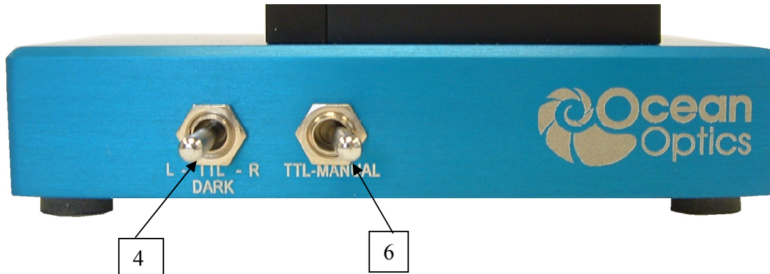
Figure 3: FOS Unit Switches
